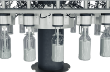
Conveying and filling The AntiSlosh function is used on machines that convey and fill containers with liquids.
