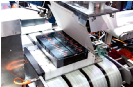
Cam-operated multipacker Side-loader design with synchronized cams and coordinated motion
