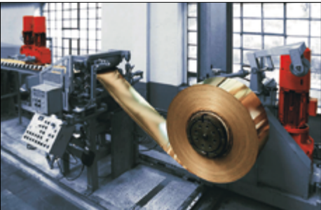
Winder in clocked machines, e.g. for stamping sheet metal
