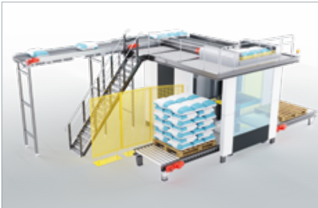
High-level palletizer Palletizer without synchronized motion (drive control)
