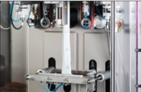
FFS machines A film is first formed into a tube, then filled, and finally sealed.
