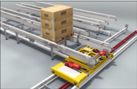
Pallet transfer shuttles – Transport systems in logistics centers
