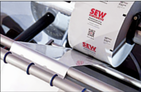
Print mark recognition Print marks, such as the black ones on this film, are used to ensure clear-cut, error-free further processing.
