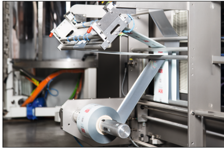
Machine with web material running through it, and with winding units and tension shafts
