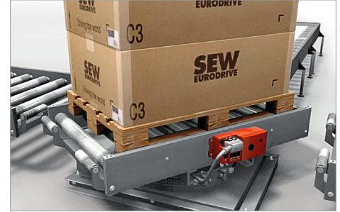
Materials handling technology with changes of direction Rotary table, carriage
