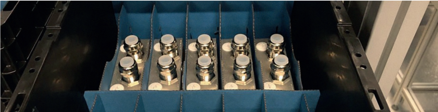
Material supply in shuttle crate without individual packaging
