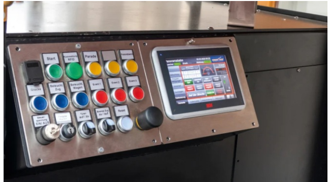
Control panel with display for operating the locomotive
