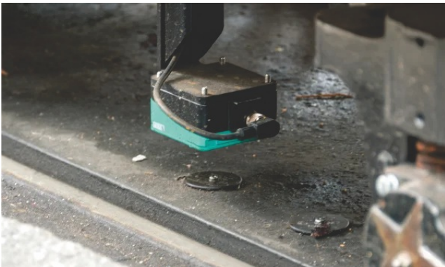
RFID sensor for positioning above the field plate
