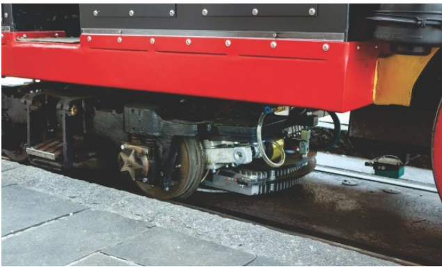
Energy transfer from field plate to TDM80E pickup
