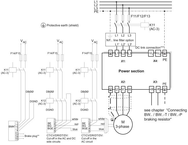
CT/CV, CM71 ... 112: Cut-off in the DC and AC circuits
