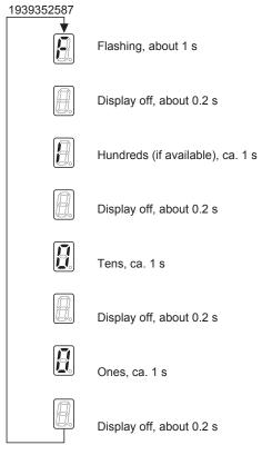
Following a reset or if the fault code resumes the value "0", the display switches to the operating display.
