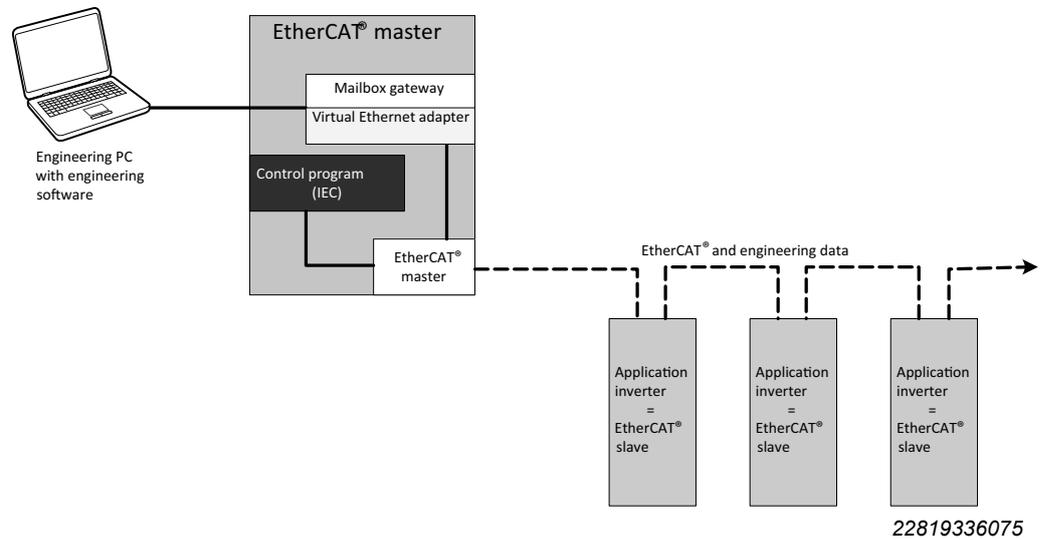
This profile is primarily used for startup of a motion axis on an EtherCAT® master and facilitates the integration of the inverter due to the standardized interface.
