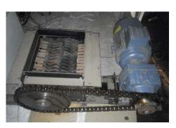
inline type gear motor units were employed. The machines have used R37, R47, R57, R67, R77 and R97 with various motor power and gear ratio combinations.
