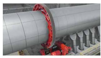
The Segmented Girth Gear (SGG) application installed by SEW-EURODRIVE at the Pellet Plant of Godawari Power & Ispat Ltd. is a mega project that can offer significant new benefits for the steel and cement industries of India. The 14-segment tension spring type SGG, fitted in the Pellet Plant kiln, generates big savings on lubrication (up to Rs. 10 lakh per year), along with reduced maintenance costs and downtime.
