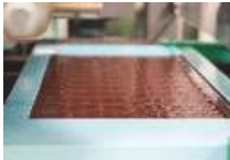
Shaken in the mold – the uniform structure of the chocolate mass leads to high product quality without air pockets
