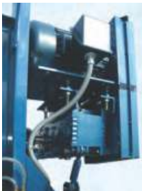
SEW custom configured an MC Compact heavy-industrial gearbox for Marion Mixers' pigment and wood chip blending system.
