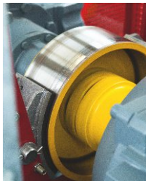
The brake brings the 75 kW drive safely to a stop.
