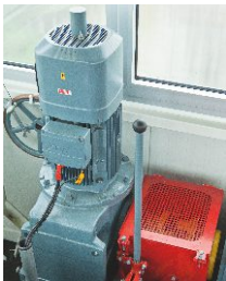
The auxiliary drive is an AC asynchronous motor from SEW-EURODRIVE with a second shaft end.
