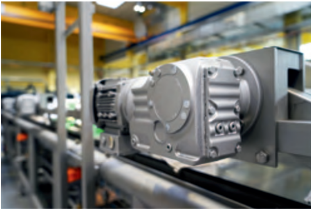
Gearmotors from SEW-EURODRIVE drive a continuous tempering unit for processing soft and hard candy mass.
