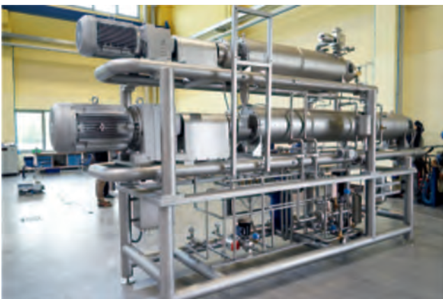
SEW-EURODRIVE gearmotors drive the tableting rotors of the MICRON continuous tableting machine.
