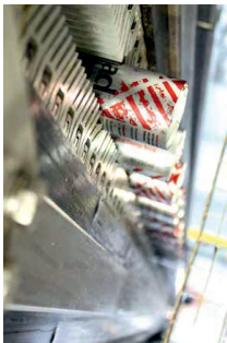
In the vertical conveyor, two parallel chains with rubber flaps gently clamp the cans and convey them upward. (Photo: Ennstal-Milch)
