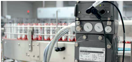
The Movigear mechatronic drive system from SEW-EURODRIVE is used for hygienic and energy-efficient transportation of the drinks packages. (Photo: Ennstal-Milch)
