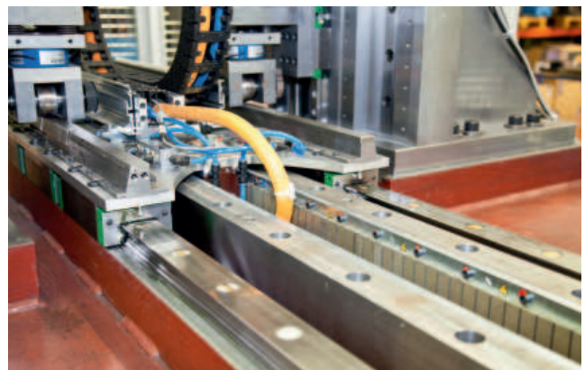
The linear drive achieves speeds of up to 6 m/s. The necessary feed thrust is provided by the rotor current. The high torque and power levels required generate heat, which makes water cooling necessary.
