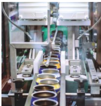
Side clamping belts are used for all kinds of purposes, for example as a feed guide for turning systems or to apply a code to the bottom of products.
