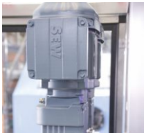
SEW-EURODRIVE motors drive side clamping belts that are used for all kinds of purposes, for example as a feed guide for turning systems or to apply a code to the bottom of products.
