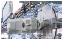
A MOVIGEAR® mechatronic drive unit drives the CA M/LOW cable transport system via the pulley.
