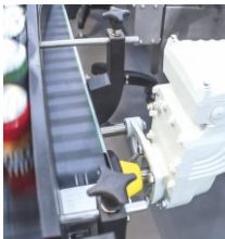
The link-belt conveyors are driven by highly efficient MOVIGEAR® mechatronic drive systems.
