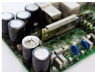
Forming helps to prevent capacitor explosions
