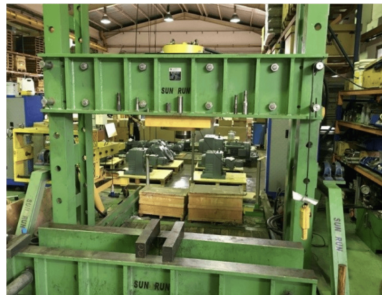
150Tons Hydraulic Press for gear & bearing removal
