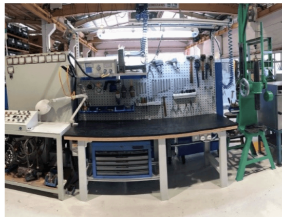
Repair workstation c/w press, test run, high potential testing panel & oven
