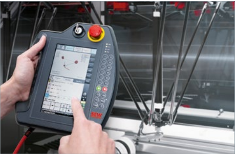
Usage Handheld device for controlling a kinematic model with the RobotMonitor for MOVIKIT® Robotics.
