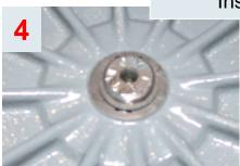
Re-install the snapring using the snapring pliers.
