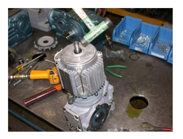
Install the fan using gentle taps with the dead blow hammer.
