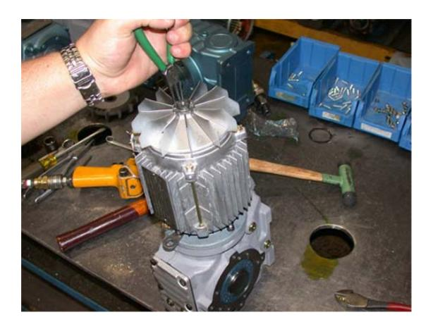
Place the fan guard over the fan, lining up the fan guard holes with the holes in the end shield.
