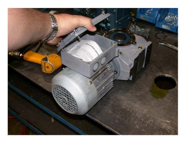
Disconnect the power wires from the motor.
