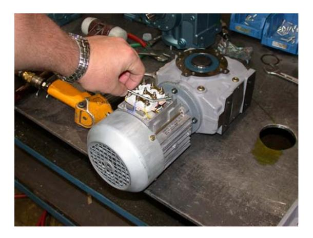
Using a metric nut-driver, remove the 4 small screws that hold the fan guard in place.
