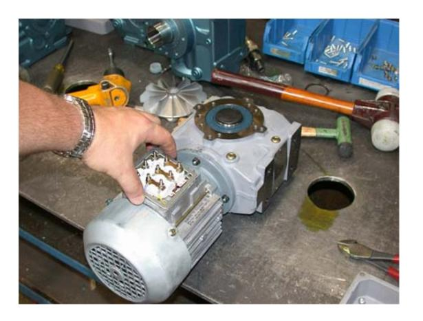
• Using the four (4) Torx screws and Torx driver, install the conduit box into its previous location to ensure that any drain holes remain in their proper position.
