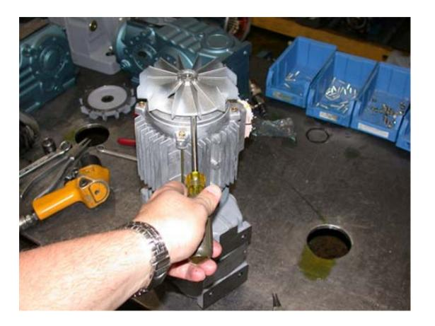
Using the cutting pliers, remove the A-key from the rotor shaft.
