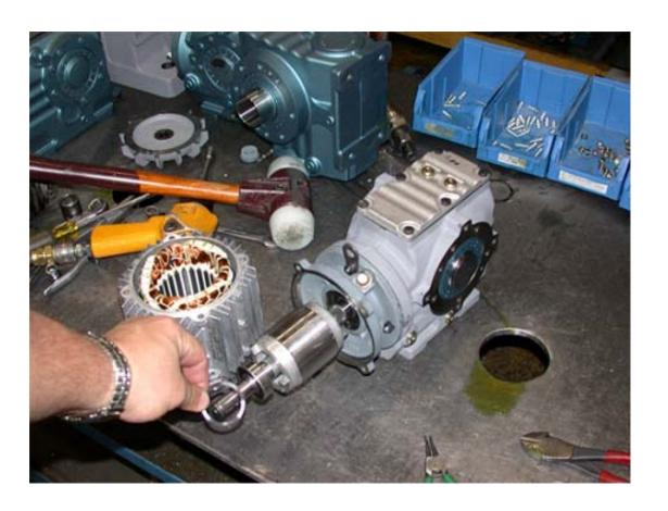
Tap the inside of the motor end shield to gently remove it from the stator.
