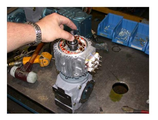
Place the motor end shield onto the rotor while keeping the wavy washer aligned. Rotate the end shield until the tension rod holes are aligned and tap the end shield into place.
