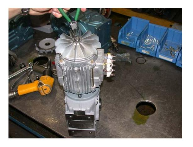
With the medium-sized flat-tip screwdriver, gently pry the fan up and down to loosen and remove it. Use caution to avoid damaging the fan!
