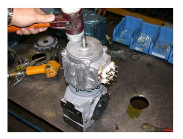
Using the appropriate metric socket and driver, install the four (4) motor tension rods.
